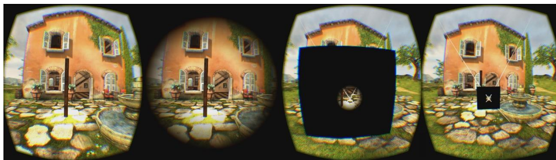
Fig. 2-1 Combating VR sickness through subtle dynamic field-of-view modification [10]
