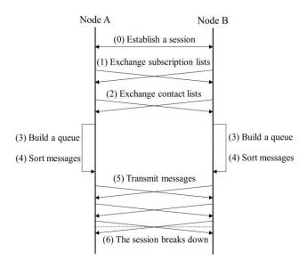
Figure 4: Communication process between two nodes
