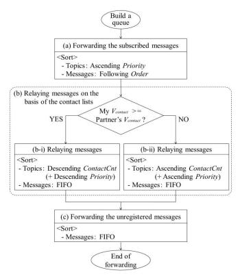
Figure 5: Procedure of forwarding messages
