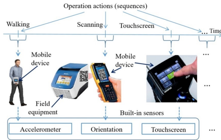
Figure 3.2: The process of raw sensor data collection during the user routine work process in IIoT scenarios.
