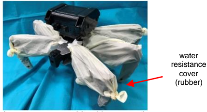
Figure 14. The hexapod robot KMR-M6 with water resist cover.
