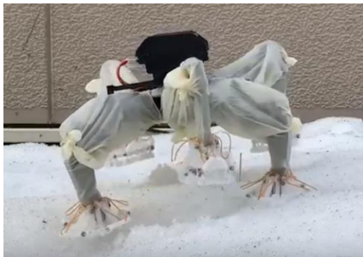
Figure 2. A multi-legged robot attached with the foldable snow shoes introduced in this paper.
