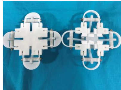
Figure 18. An original shoe with framings (right) and the shoe for the comparison which is covered by flat plates at the bottom (left).
