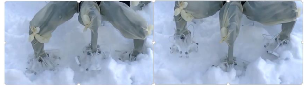
Figure 17. Passive fold and extension of the shoe in the experiment on the soft snow.
