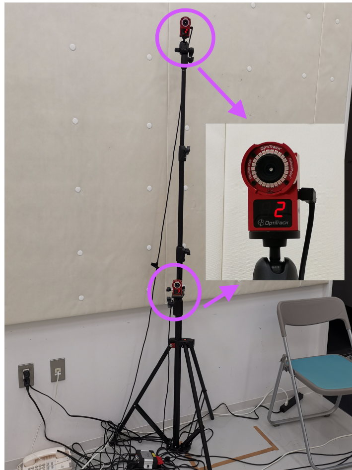
Figure 3.3: Two OptiTrack Flex 3 Cameras were Installed on One Camera Stand at Different Height Levels
